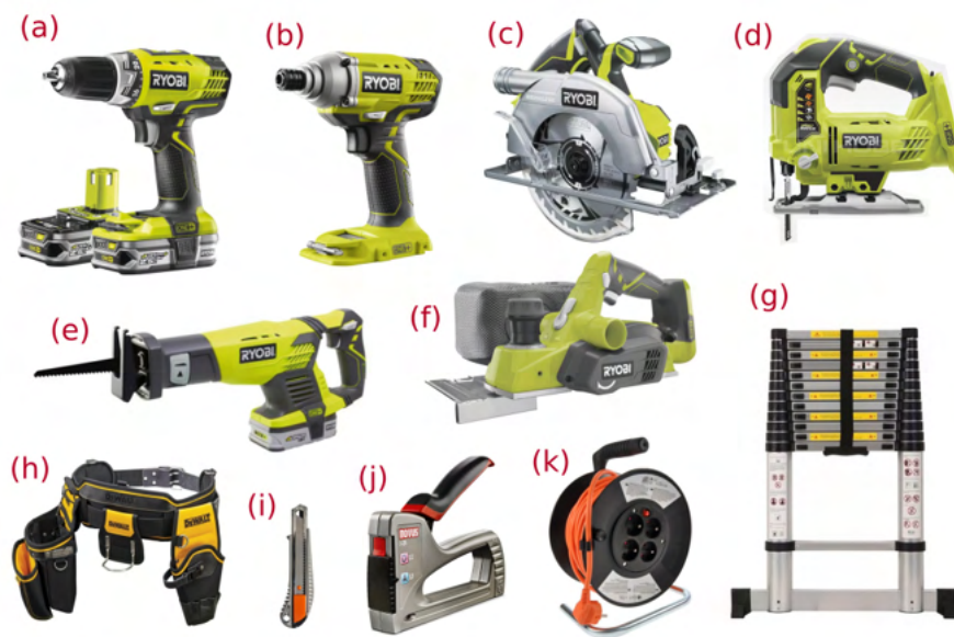
Fig. 3.5: Necessary tools. A cordless drills are essential for pre-drilling and screwing (a,b). Different types of saws for adjusting the dimensions of boards — circular (c); straight line (d); tail (e). Bevel plane (f). Folding ladder for access to elevated places (g). Other small tools for greater work efficiency (h–k).
